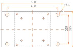
Avoids toppling or displacement of the load with the ground fixing system Protects the load cell against side forces and impact loads Eliminates problems arising from thermal expansion
